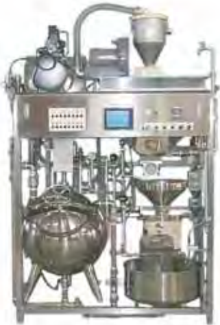
豆の浸漬→すりつぶし→煮沸 Dip → Grinding → Boiling
