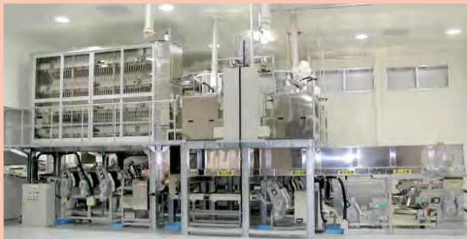
Completely automated equipment 6,000 to 15,000 servings/hour
